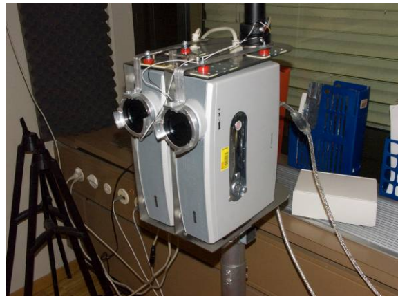
Figure 4: Dual-projector assembly with shutters.
